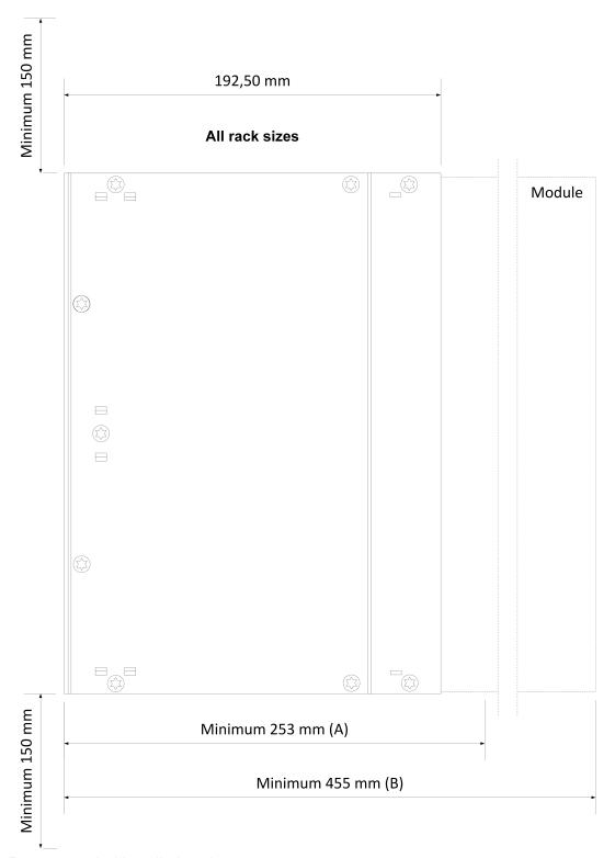
Figure 2. Recommended installation clearance.
